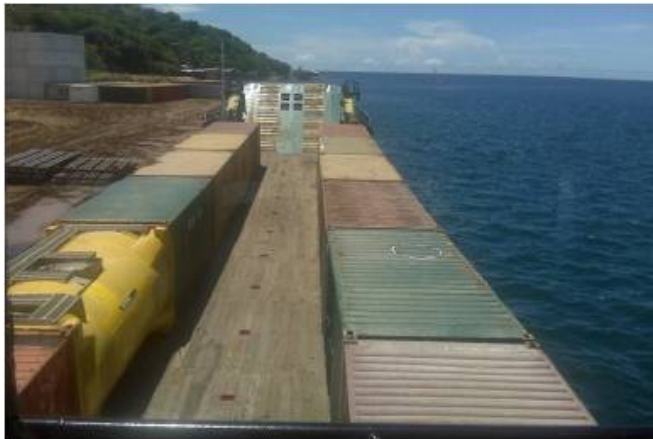
Ramp Door: 6.7 m (length) x 8 m (width) Can load up to 18 x 20 ft containers
